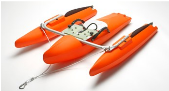
TELEDYNE RDI RiverRay ADCP (600 kHz phased array).
