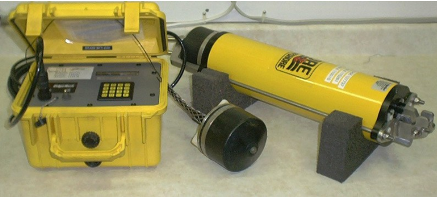
EdgeTech Model AMD200R acoustic deck unit and similar EdgeTech PACS LF acoustic deck unit.
