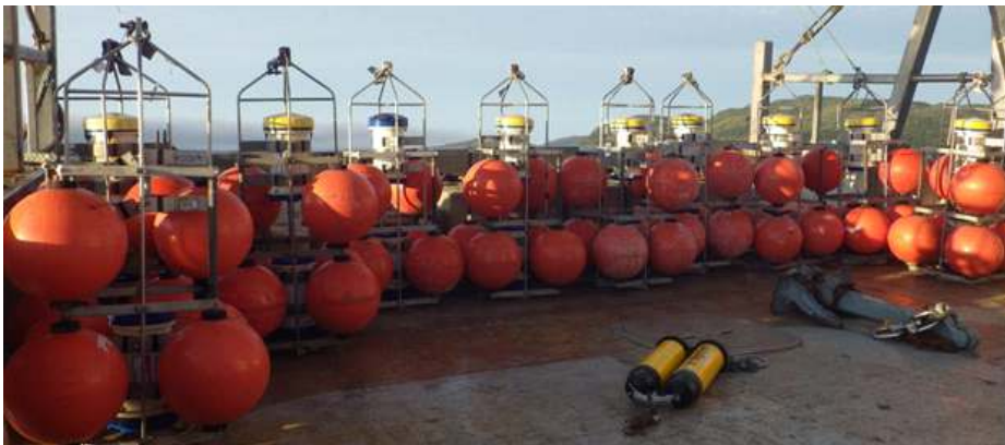
Ten taut-line current meter moorings ready to deploy for a major aquaculture company. Most of the moorings had both upward- and downward-looking ADCPs, allowing full water column current profiles, including near-surface and near-bottom.
