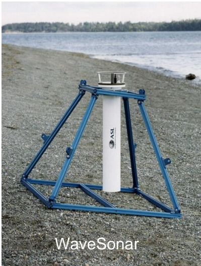
FIGURE 4: Photograph of the upward looking sonar (WaveSonar) instrument as well as the mounting frame, prior to deployment. The WaveSonar was used for ship wake waves measurements at the 68 m deepwater measurement site.
