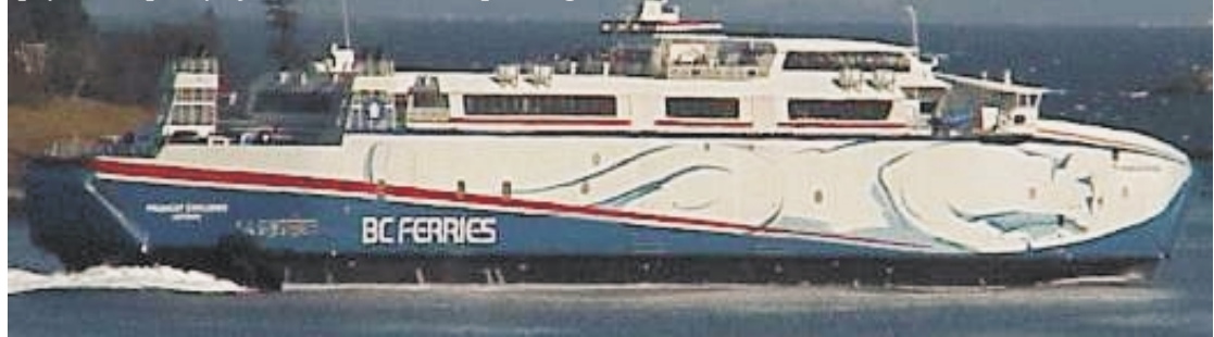
The PacifiCat Ferry, a 400' long catamaran hull having a maximum speed of 37 knots, with a payload capacity of 250 cars and 1000 passengers.
