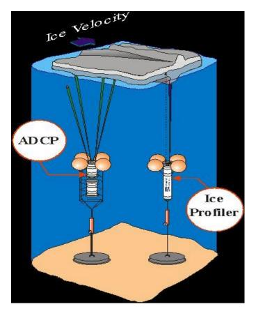
Figure 1. A typical deep-water ice profiling site with Ice Profiler and ADCP instruments deployed on adjacent, independent, moorings. The instruments are typically deployed at depths of 30 to 100 m in total water depths of 30 to 200m.
