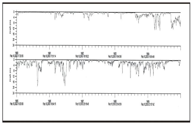
Figure 2. A plot of ice draft along a linear ice cover track in the Sea of Okhotsk.
