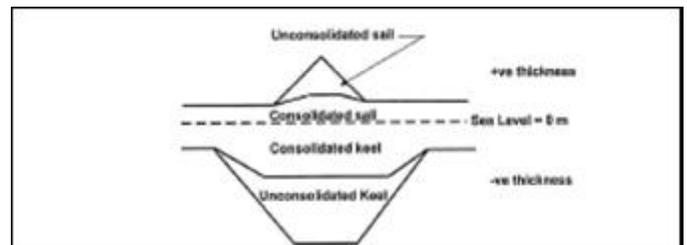
Figure 6: Actual Ice Profiler keel features, such as those shown in Figure 2, can be fitted to idealized geometry with characteristics as shown.
