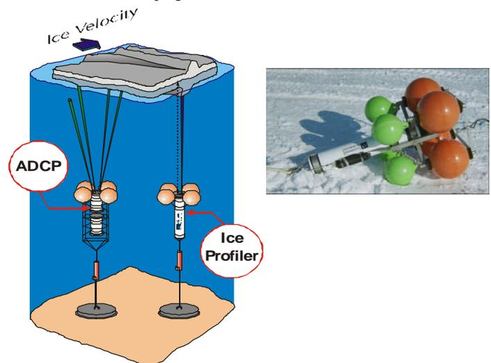
Figure 1. A typical deployment arrangement of an ice profiler and ADCP ice velocity measuring instruments on separate, sea floor-based, moorings.
