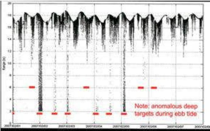
Figure 10. Raw ranges of “first targets” detected over a week-long monitoring period with the IPS5 instrument in Northumberland Strait (from Fissel et al., 2007).
