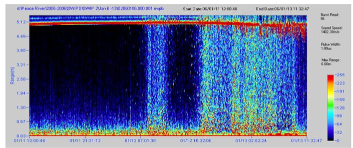
Figure 9. Acoustic target strength profiles gathered over a 2 day period in about 5 m of water in the Peace River during an interval which included two major intervals of frazil ice production by extreme atmospheric cooling. The downward-extending strong (Red) target strengths at the upper ends of the profiles in the latter half of the record correspond to returns from ice floes drifting downstream over the monitoring site.
