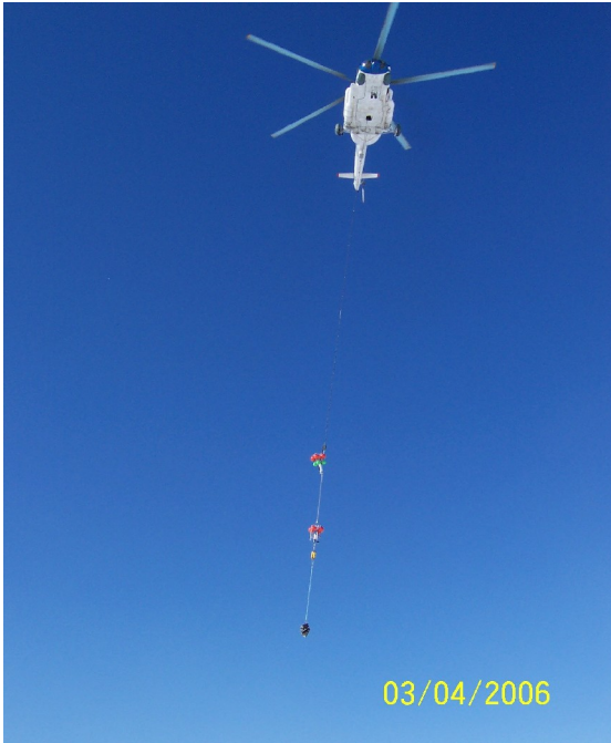
Fig. 7. Helicopter-borne deployment of an IPS4 +ADCP mooring (BP Ltd. Photo).
