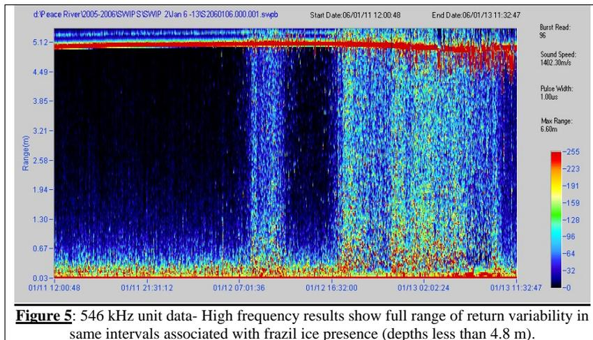
**Figure 5:** 546 kHz unit data- High frequency results show full range of return variability in same intervals associated with frazil ice presence (depths less than 4.8 m).
