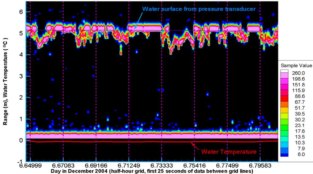
**Figure 2 Dec. 6, 2004 SWIPS1 25 1-second resolution profiles are plotted data for successive half hour intervals as denoted by vertical grid lines. Ice floes and frazil point reflectors are evident as are plots of water temperature and water level data.**
