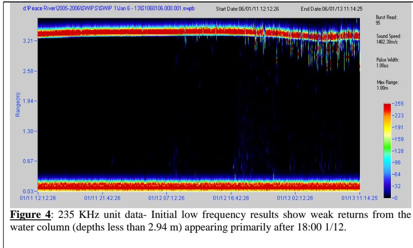
**Figure 4:** 235 KHz unit data- Initial low frequency results show weak returns from the water column (depths less than 2.94 m) appearing primarily after 18:00 1/12.
