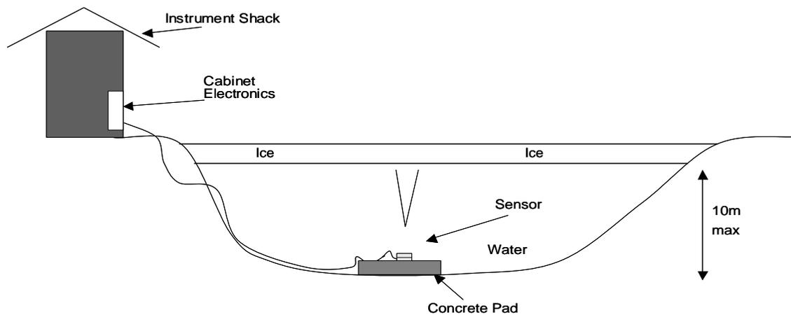
**Figure 1. Sketch of Peace River test deployment configuration.**
