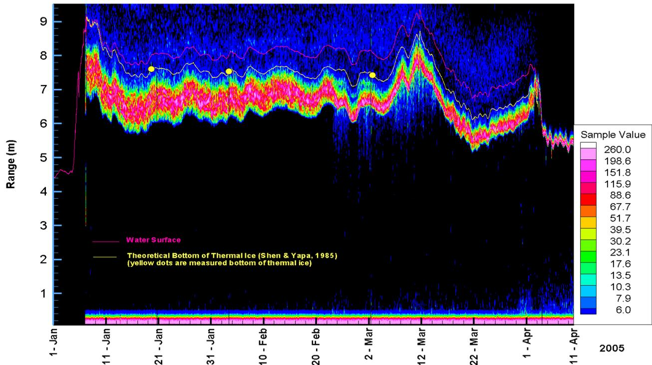
**Figure 3 Hourly profiles for mid-winter stationary ice covered period Jan. - Apr. Thermal break-up occurred on Apr. 3. Also shown are local water levels and positions of the modelled, and measured (on 3 dates) bottoms of the thermal ice.**
