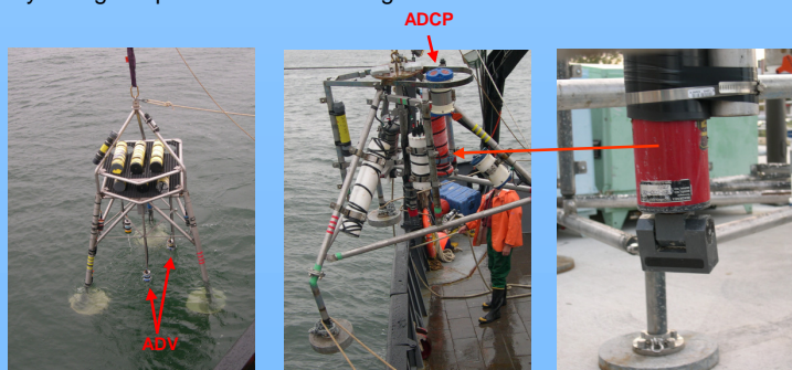
Figure 2. Instrument tripod at site 7 with ADV sensors installed on it.
