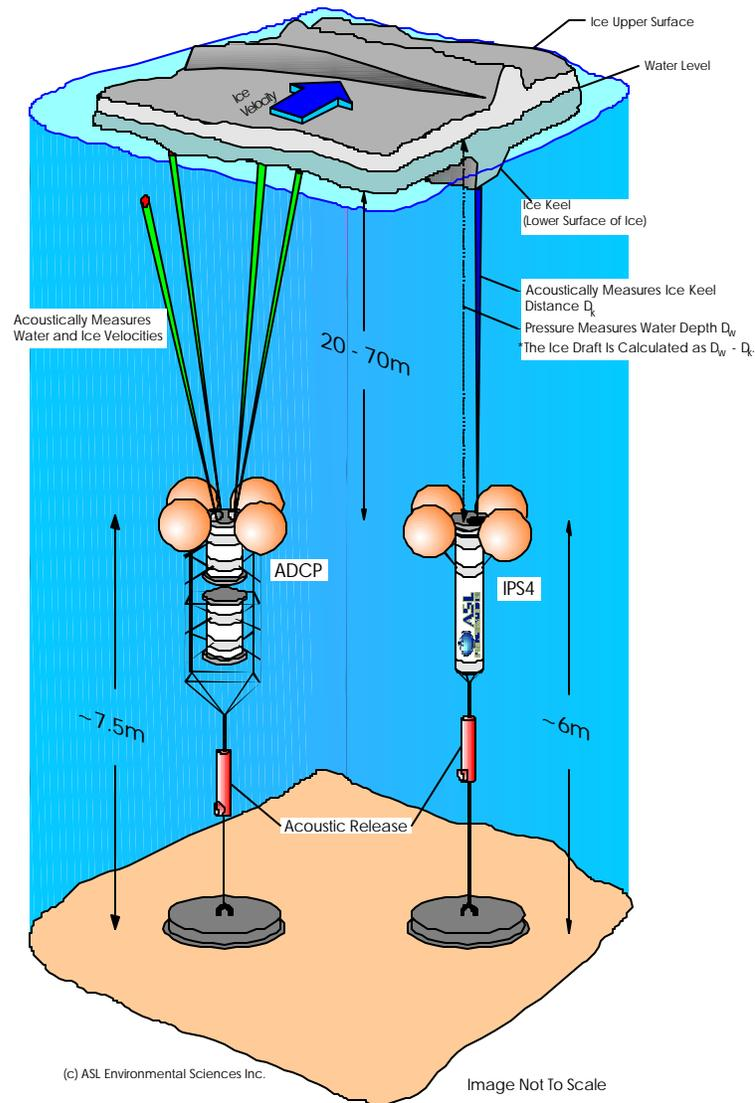
Figure 2. Mock-up presentation of the moored instrumentation used to measure ice keel depths (IPS4) and ice velocity (ADCP).
