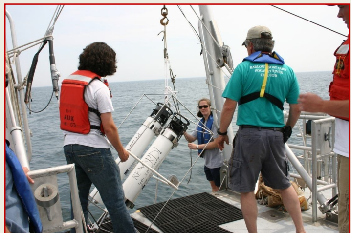
Dr. Miksis-Olds deploying a mooring containing 3 AWCPs in Cape Cod, MA courtesy Dr. Miksis-Olds
