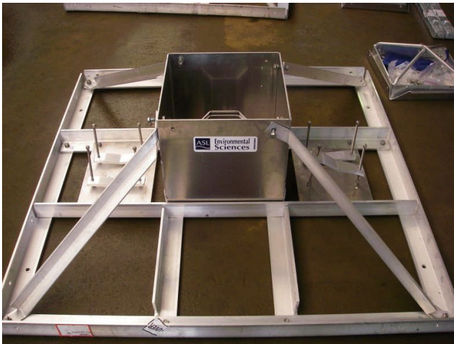
Figure 9: The low profile aluminum bottom frame for Ice Profiler Sonars as used in the NE Caspian Sea.
