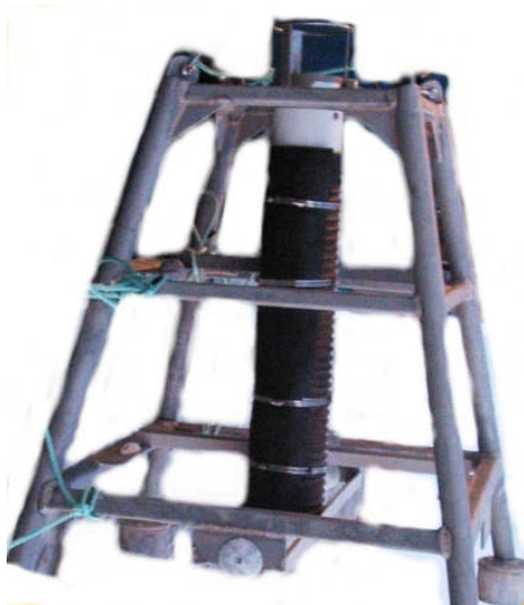
Figure 7: Ice Profiler Sonar model IPS5 mounted on a bottom mooring.
