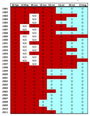
For the NE Baffin Bay AOI, potential ship passages (Table 2) were only possible starting in mid-July during most of the 1980's and 1990's. However, there is a distinct trend towards earlier potential ship passages starting in 1998. This change in potential ship passages is consistent with the changes in overall sea ice conditions noted in the previous section.
