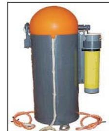
**Oceanetics Measurement Ltd pinger receiver.** In collaboration with OML, we have developed a multi-frequency pinger receiver (27, 37 and 45 kHz). The omnidirectional hydrophone sends the signal to headphones and a large speaker on the deck box. This receiver was developed specifically to listen to tilt-pingers to ensure that bottom frames are deployed upright.
