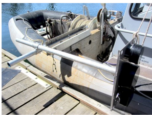
Figure 2: The transducer mount swivels to allow the transducers to be lifted out of the water.
