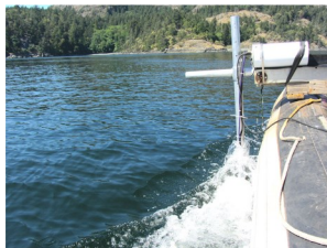
Figure 3: Collecting data at 4 knots (7.5 km/hr) without interference from bubbles.
