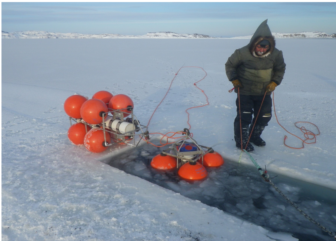
Joey Angnatok preparing ADCP and IPS mooring cages for deployment through the ice. (Photo credit: James Barlett)
