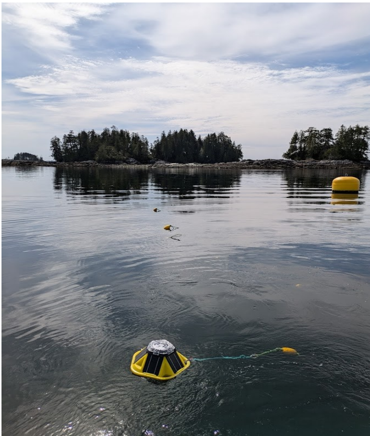
Smart AZFP-nano equipped Spotter Buoy deployed at the West Coast Kelp farm in Barkley Sound.
