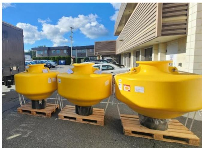
**Figure 2.** ASL has received three yellow buoys (the standard cautionary buoy colour) and are instrumented with a yellow flashing light to conform to the standards and guidelines in the Canadian Aids to Navigation System (TP 968).
