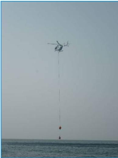
ASL's subsurface moorings were deployed/recovered by helicopter, ship, and small vessel over the 5 trips spanning the 12 month project. (Initial deployment, recovery-service-redeployment, and final recovery).
