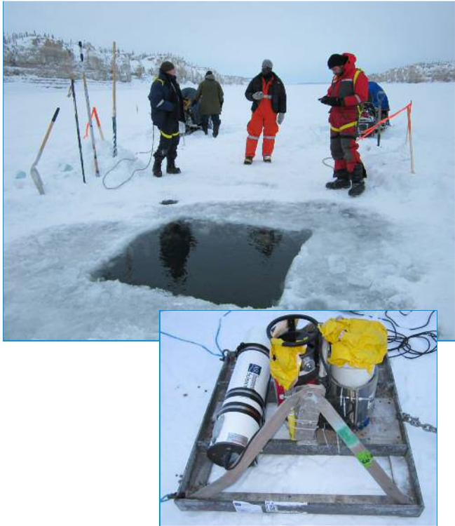
**Preparation of bore-hole for deployment of ice and current profiling equipment through the Mackenzie River ice cover.**
