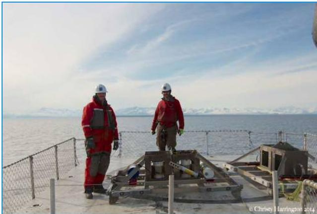
Later in October, the 8 moorings were replaced with four custom-built heavy duty frames each containing an Ice Profiler, ADCP, CT and OBS (see Figure 1). ASL will return to the sites biannually to download data and service the moorings.
