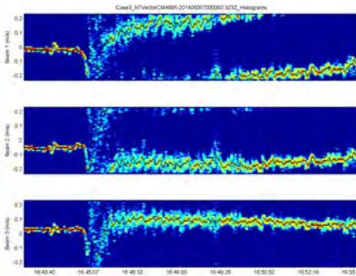
ASL developed a method to quickly identify turbidity events within the huge 2 terabytes of multi-sensor data from 2012-2016. The previously unusable Acoustic Doppler Velocimeter data from the events were analyzed with a unique algorithm.
