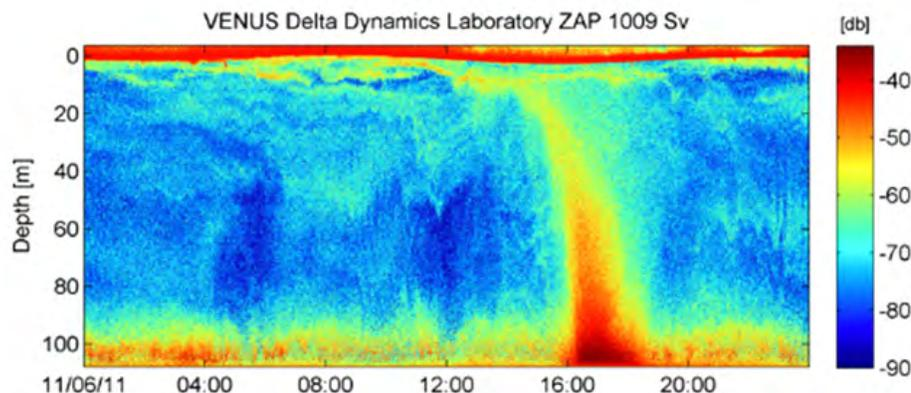
Ocean Networks Canada has been operating ASL's upward looking sonars since 2007 on the Venus network. One of ASL's instruments, a single frequency 200 kHz sensor, was deployed in 100 m of water at the mouth of the Fraser River, Vancouver at their Delta Dynamics Laboratory. It was deployed to view sediment distribution.
