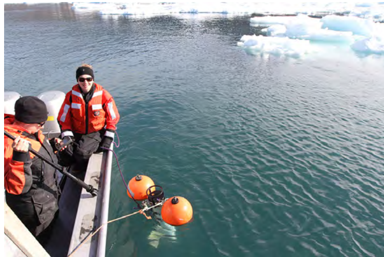
Figure 2: Sarah Fortune with 4-frequency AZFP—image taken by Dr. Bill Koski (LGL Limited).
